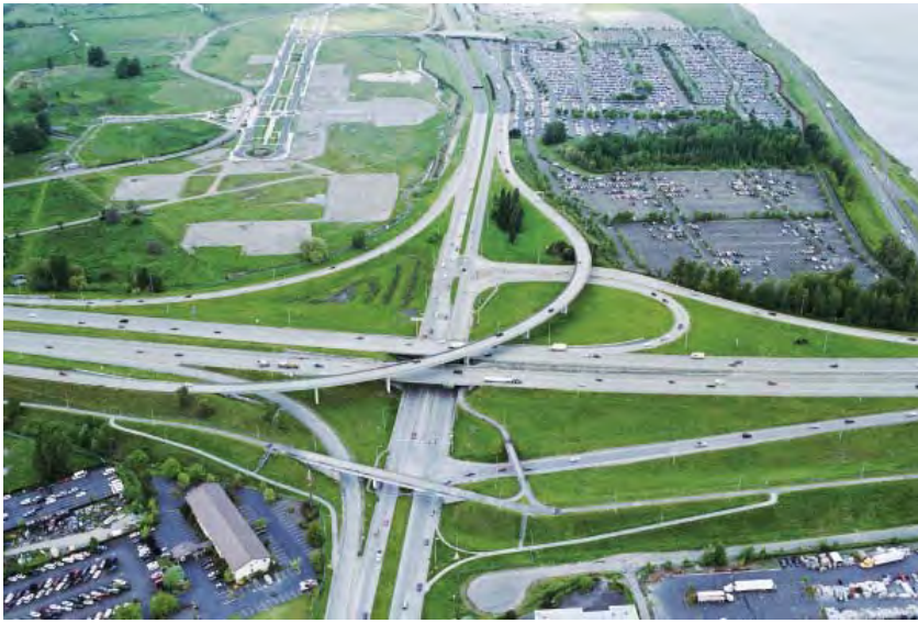
Figure 10-40. Four-Leg Interchange, Diamond with a Direct Connection
