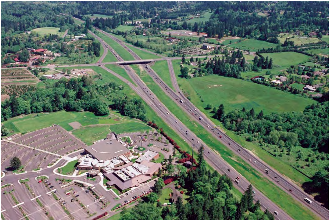
Figure 10-16. Typical Four-Leg Diamond Interchange
