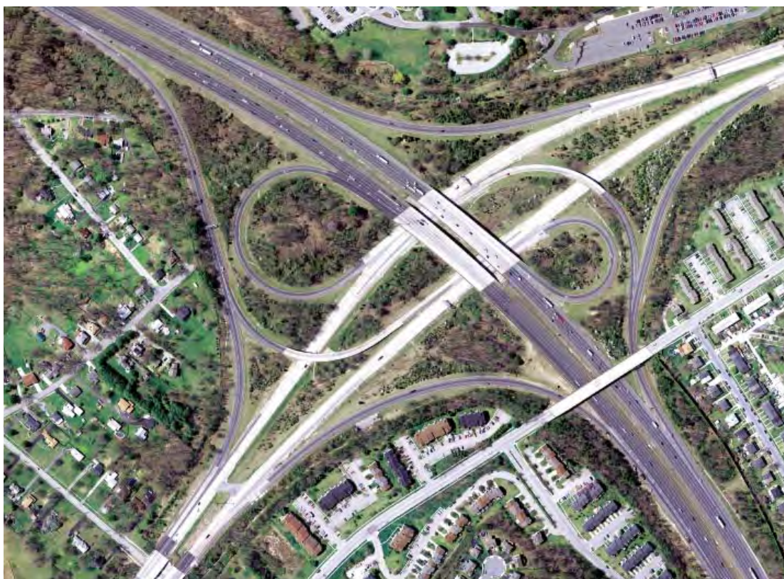
Figure 10-38. Directional Interchange with Semidirect Connection and Loops
