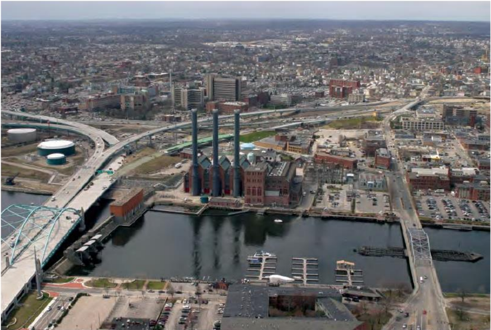
Figure 10-13. Directional Three-Leg Interchange at a River Crossing
