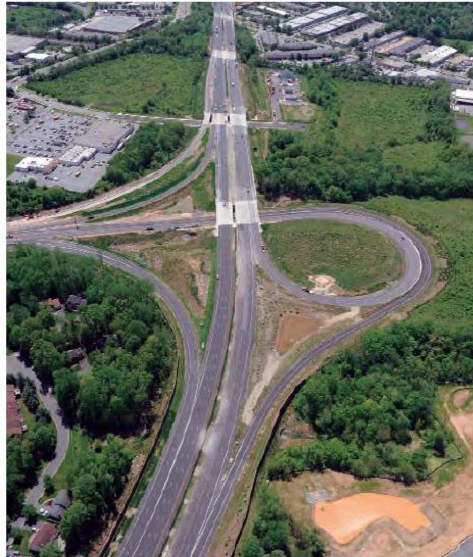
Figure 10-14. Trumpet Freeway-to-Freeway Interchange Source: Maryland DOT
